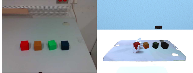
Fig. 7: The scenes in Fig. 5 were generated from longer SLAM trajectories, whereas here, the input ConceptGraph [1] was built from a single frame captured by an Intel Realsense™ mounted on a robot arm. This scene highlights another useful aspect of PerceptTwin: the scene is quite representative of the input map, down to the raised bumps and the holes in the TRELIS-generated [27] table surface that reflect the masks left behind by SAM [13] segmentation.
